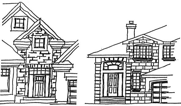
When brick is utilized as the predominant front elevation cladding material, brick returns may not be required.
