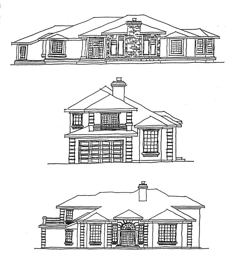
Rear and Side Elevations - The rear and side elevations must be clad with the same cladding material utilized on the front elevation except when the front elevation is entirely clad in brick, stone, or stone tile, then any one of the approved cladding materials may be utilized.
